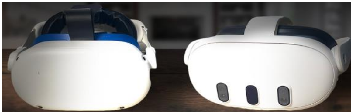
Figure 47 - The Meta Quest 2 and 3 headset devices, the primary internal sensing devices used in 6G-SANDBOX's Sensing lab at UOULU. They provide 6-DoF pose and velocity, video, audio and AR/VR Rendering. The Meta Quest 3 also offers environment depth sensing
