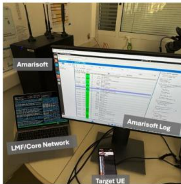
Figure 33 - Lab setup for LMF testing at the Athens Platform
