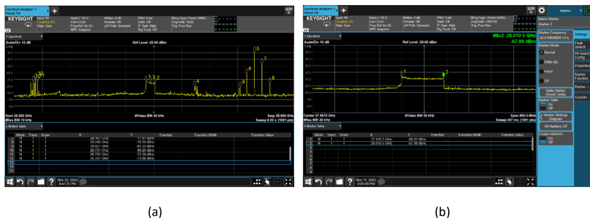
Figure 45: Measured spectrum figures (a) Wide span spectrum and (b) 5G signal spectrum
