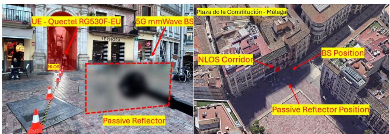
Figure 36 - Overview of the outdoor measurements using a cellular mmWave system with a Reflector to enhance connectivity in a narrow, NLoS urban environment
