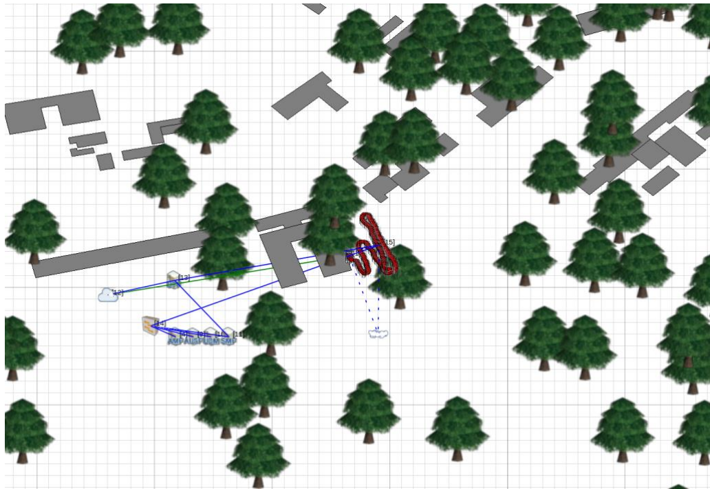
Figure 71 - Final setup of the configuration of 5G SA deployment of the EXata Digital Twin and the path taken on the NCSR Campus
